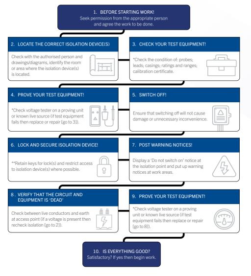
Reference should be made to the current editions of the \*Health and Safety Executive's Guidance Note GS38, Electricity at work – Safe working practices HSG85 and \*\*BS 7671 Guidance Note 2 – Isolation & Switching
